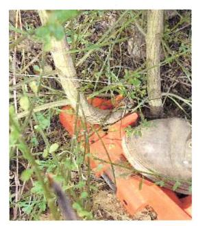
Weed Wrench is easily used by placing the jaws around a woody stem. Pushing the handle forward opens the jaws, pulling back closes the jaws. When the jaws can't close any more on a woody stem, the tool begins to rock on its fulcrum, uprooting the plant.
